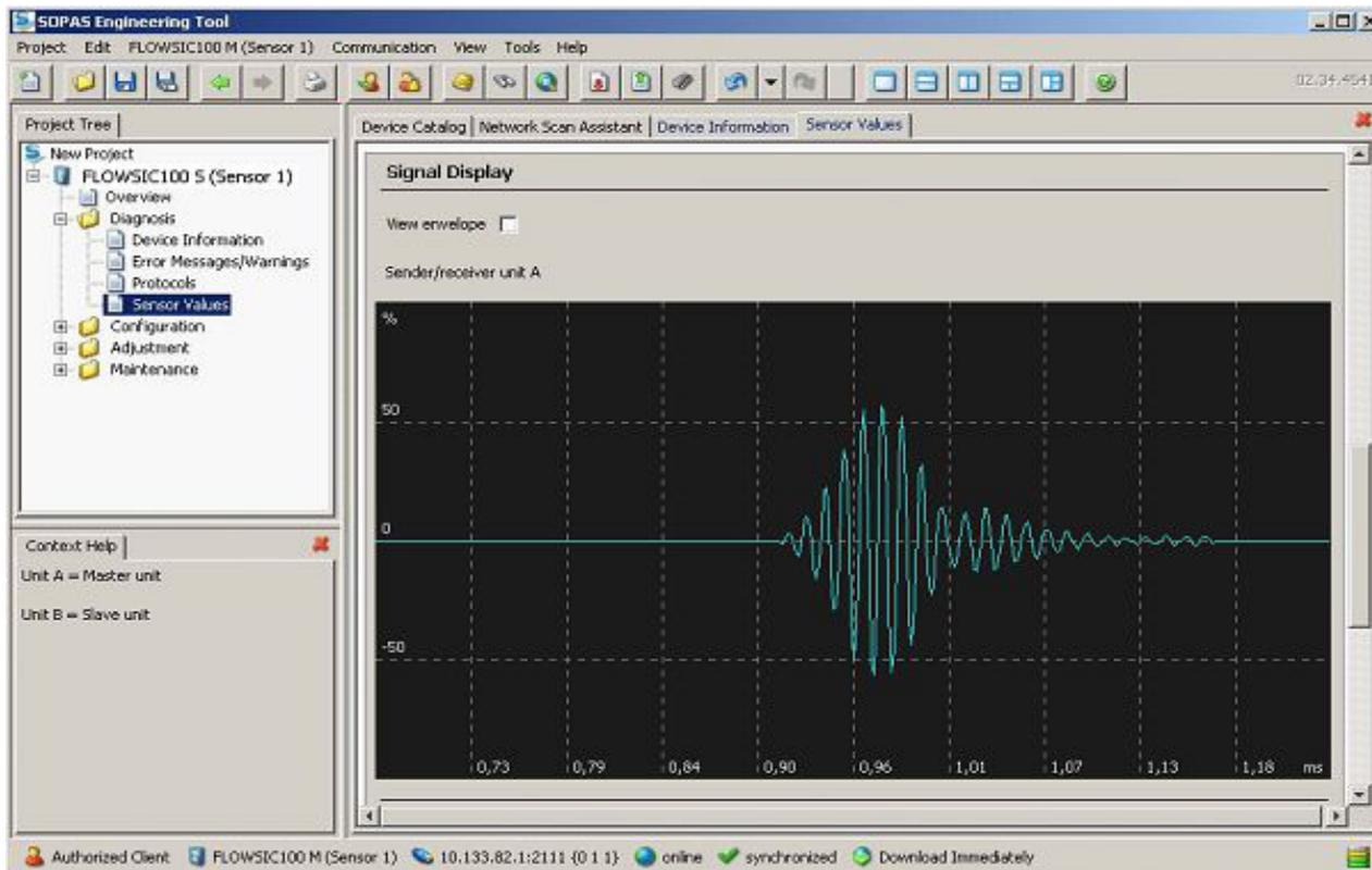
Fig. 59 Burst waveform demodulated signal (envelope)
