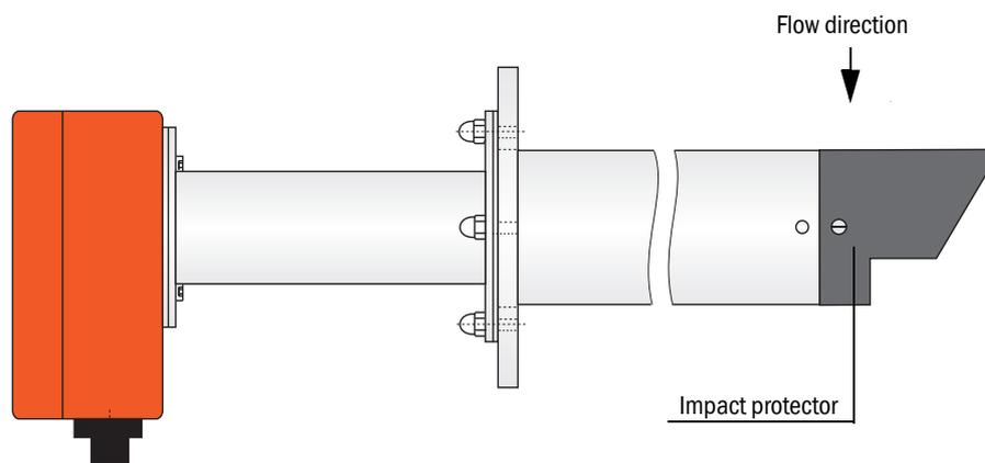
The impact protector is located on the probe head as shown in Fig. 25 and must be aligned facing the flow direction.
