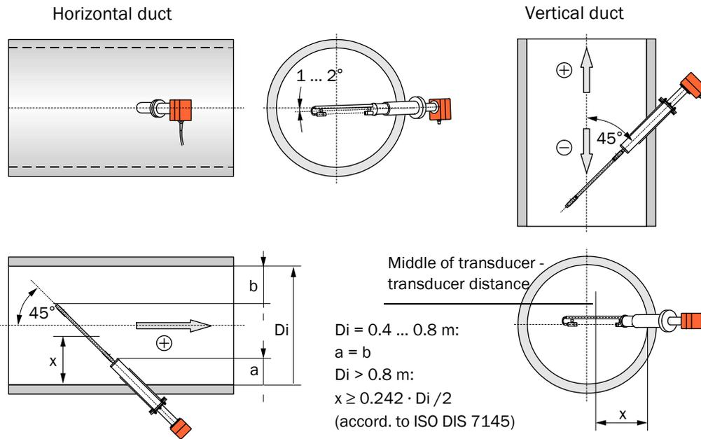
$x$  = representative wall clearance at which the local gas flow rate is the same as the mean velocity in the duct cross-section
