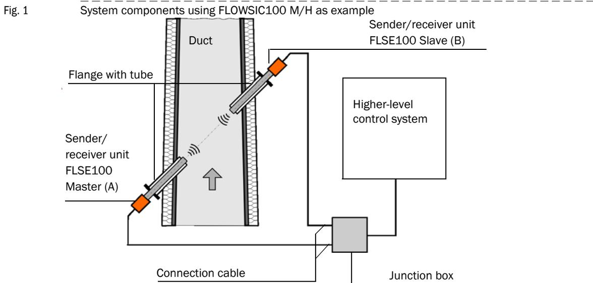
2.2.2 **Communication between sender/receiver units and higher-level control system**
