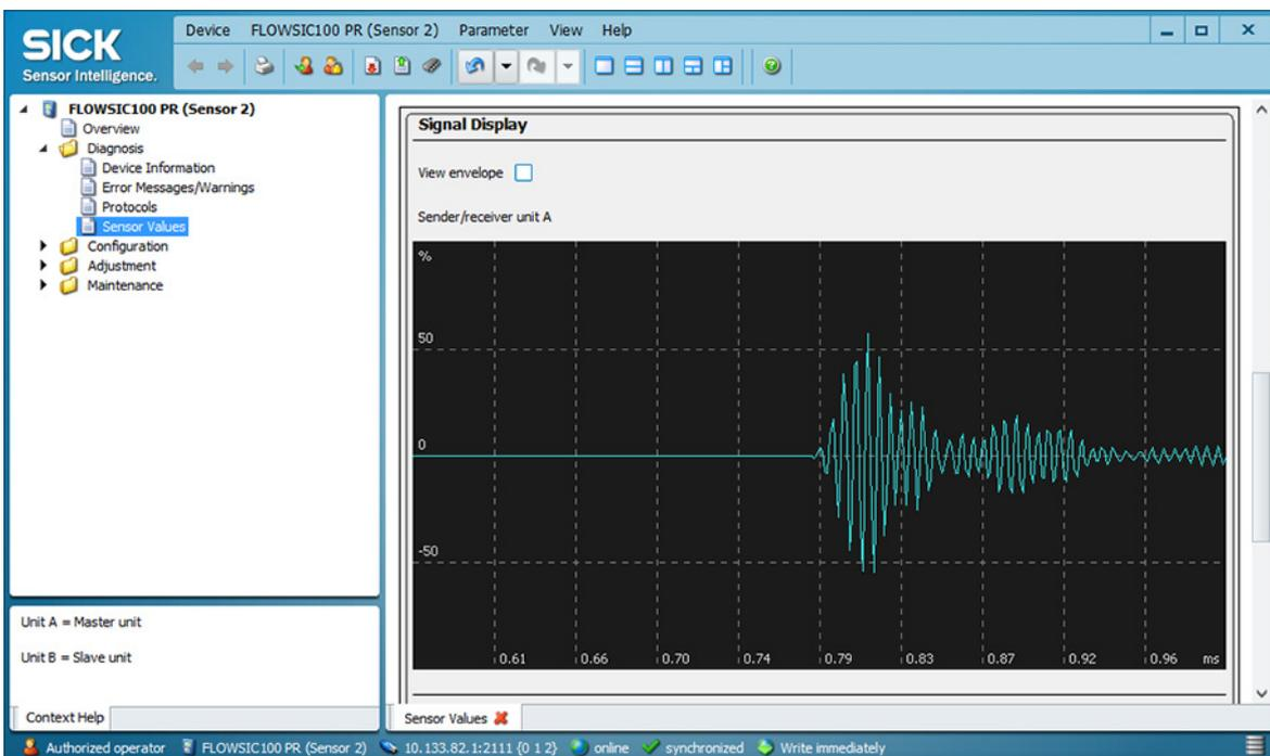
Fig. 61 Burst waveform demodulated signal (envelope)
