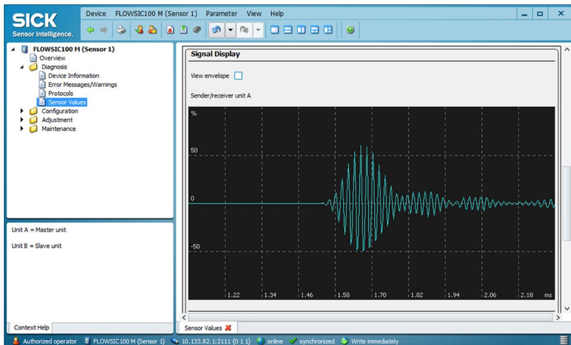
Fig. 55 Burst waveform demodulated signal (envelope)
