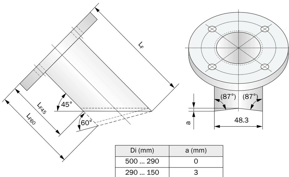
Flange tube length  $L_F$  ( $L_{F45}$ ,  $L_{F60}$ ) depends on installation angle  $\alpha$ , wall thickness  $w$  and nominal length  $NL$  ( $\rightarrow$  Fig. 22,  $\rightarrow$  Fig. 23). This correlation is expressed by the following formulas:
