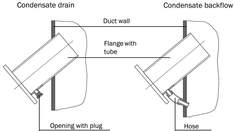
**Using the sender/receiver units with high dust contents (> 1 g/m<sup>3</sup>)**
