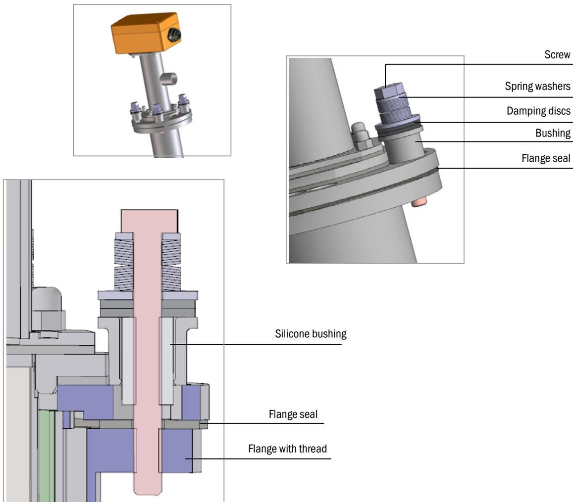
**Installation instructions for solid-borne noise damping set option K100/K75**
