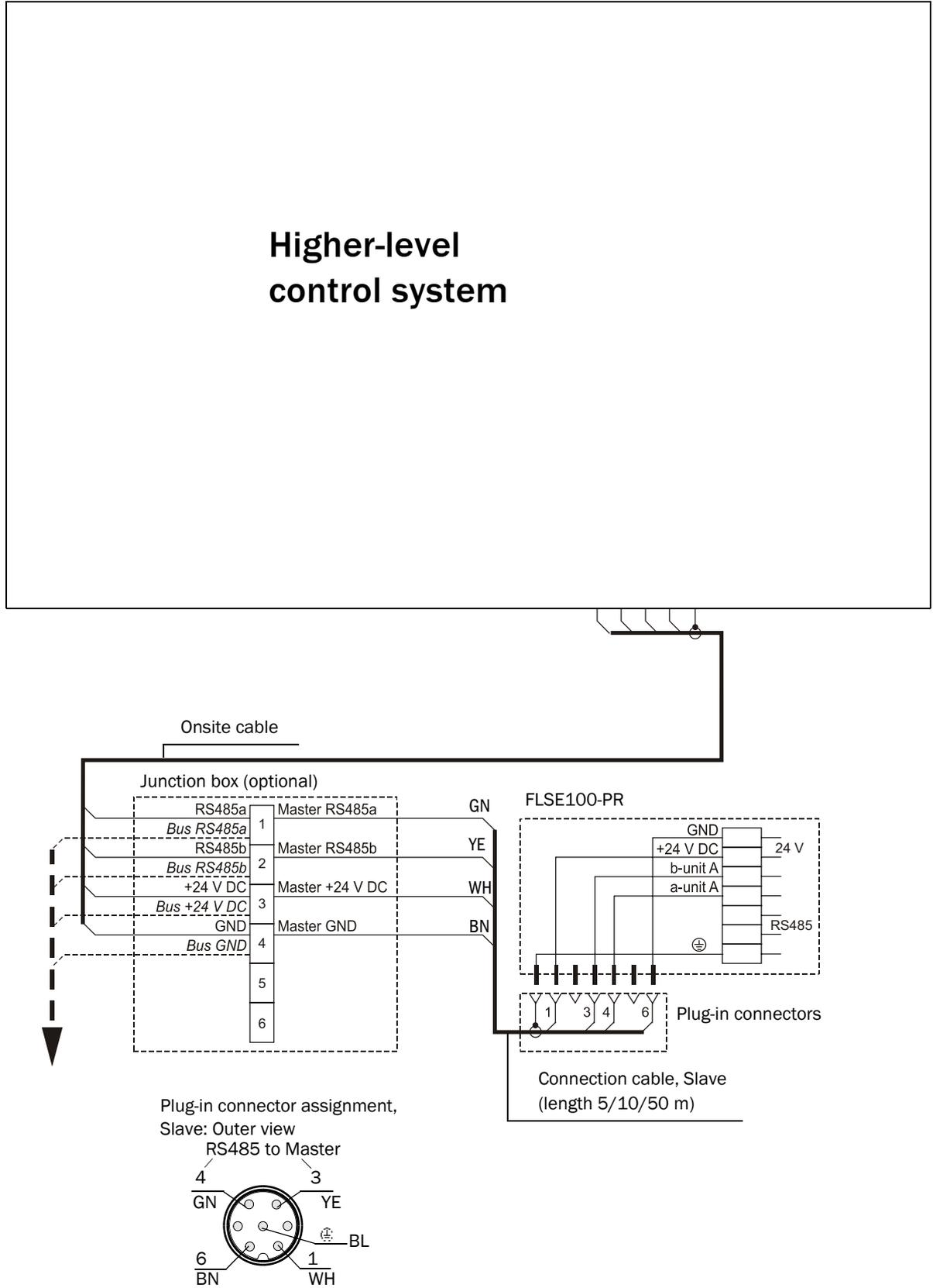
Fig. 31 Connection of the FLOW SIC100 S to the higher-level control system
