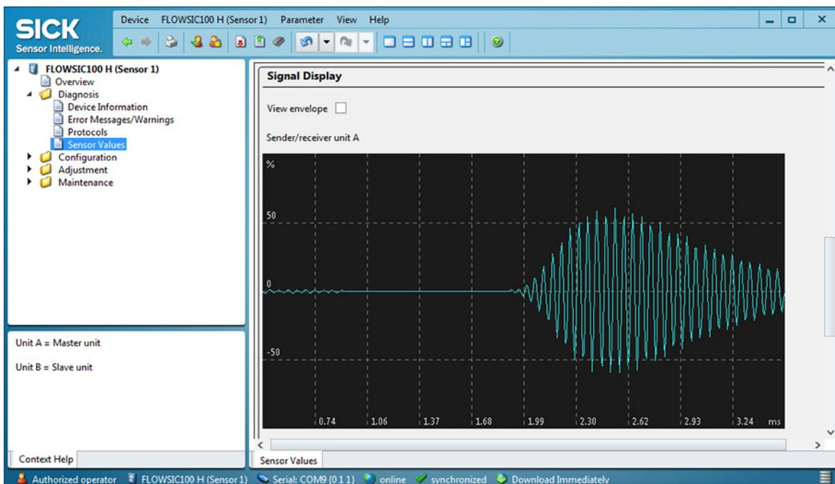
Fig. 57 Burst waveform demodulated signal (envelope)
